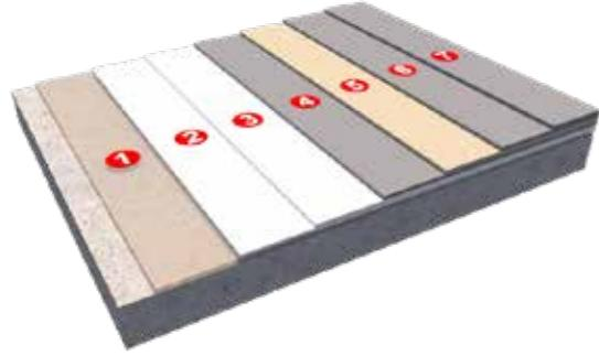
A flexible, non-slip, rapid cure hybrid PU MMA top deck waterproofing system that offers excellent crack bridging properties.
